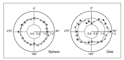
**Figure 8.2.** Cylindrical symmetry as indicated by an isotropic neutron radiation field *Note*: Ideally, if the item is cylindrically symmetrical, the neutron counts in all detectors will be equal. A test is made for a significant variation from equality according to the formula:
